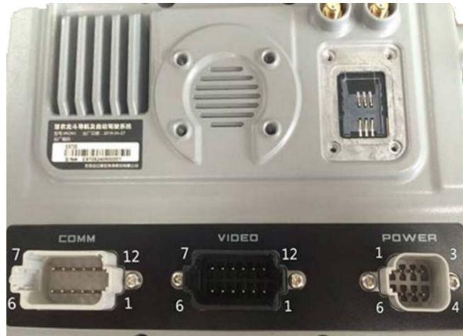
Figure B-3: IronOne pin-out assignments
