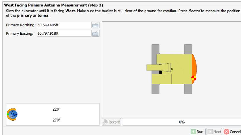
Keep the boom and bucket equipment still and record the **Primary Antenna** location using the **Record** button.
