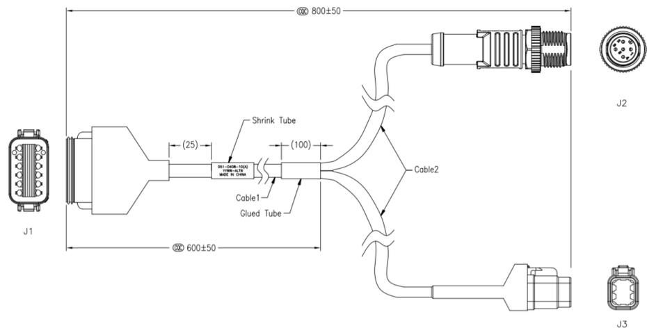
**Figure 2-3: Cable schematic for Part Number 054-0182-10**
