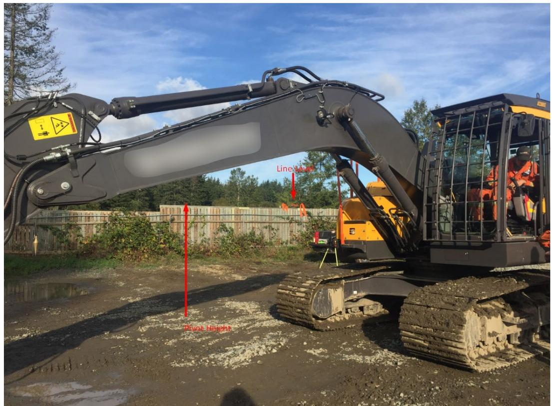
**Figure 3-2: Measuring the pivot height**
