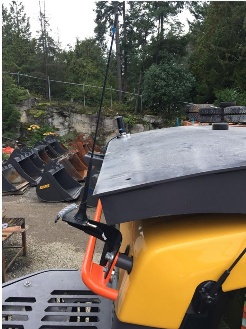
**Figure 2-12: Radio antenna**
