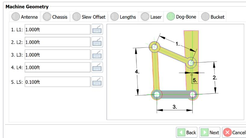
The L1-L4 measurements must be measured precisely and entered in per the diagram.
