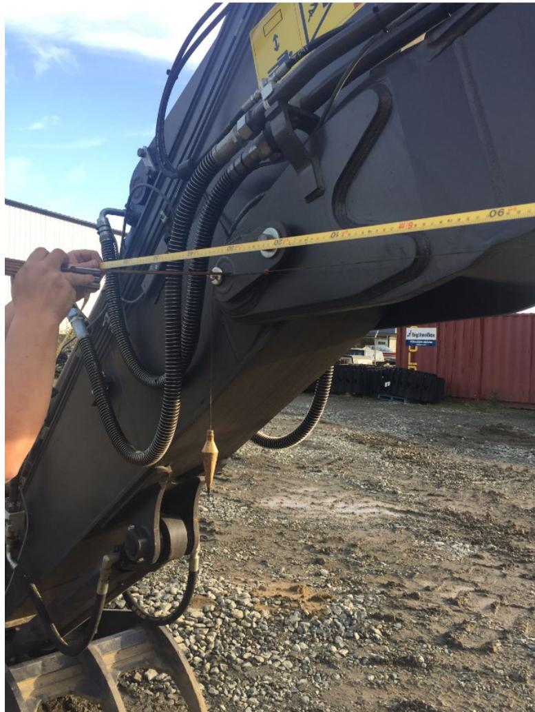
**Figure 3-3: Measuring the boom pin to stick pin**
