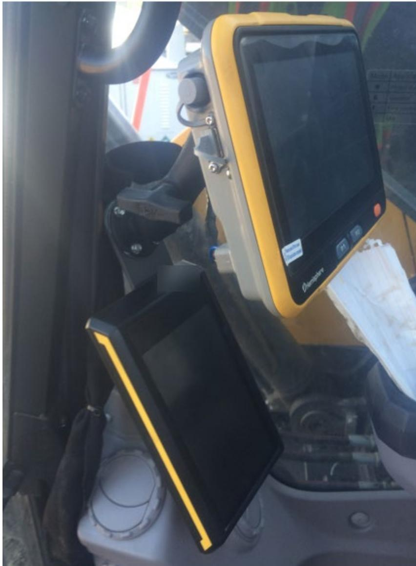
**Figure 2-2: IronOne control box-mounting option #2**
