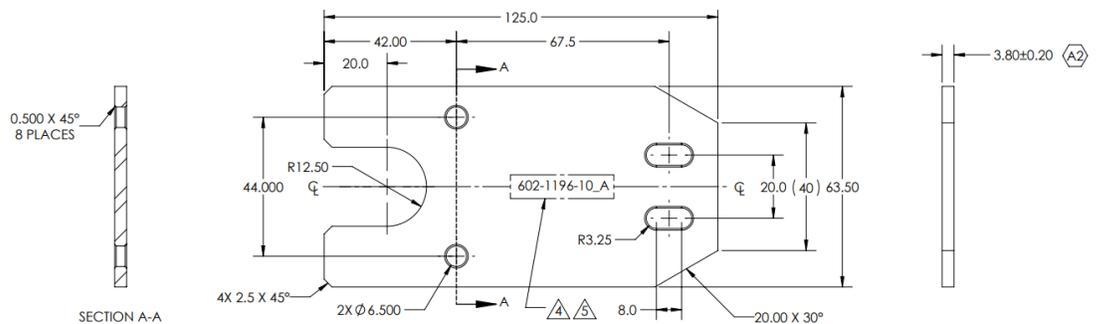
**Figure 2-6: P/N: 602-1196-10 strain relief wing**
