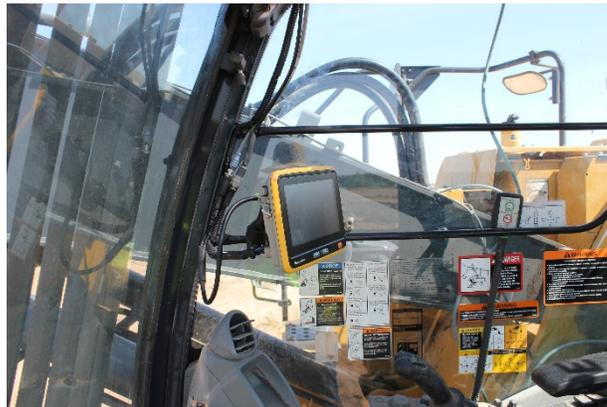
**Figure 2-1: IronOne control box-mounting option #1**
