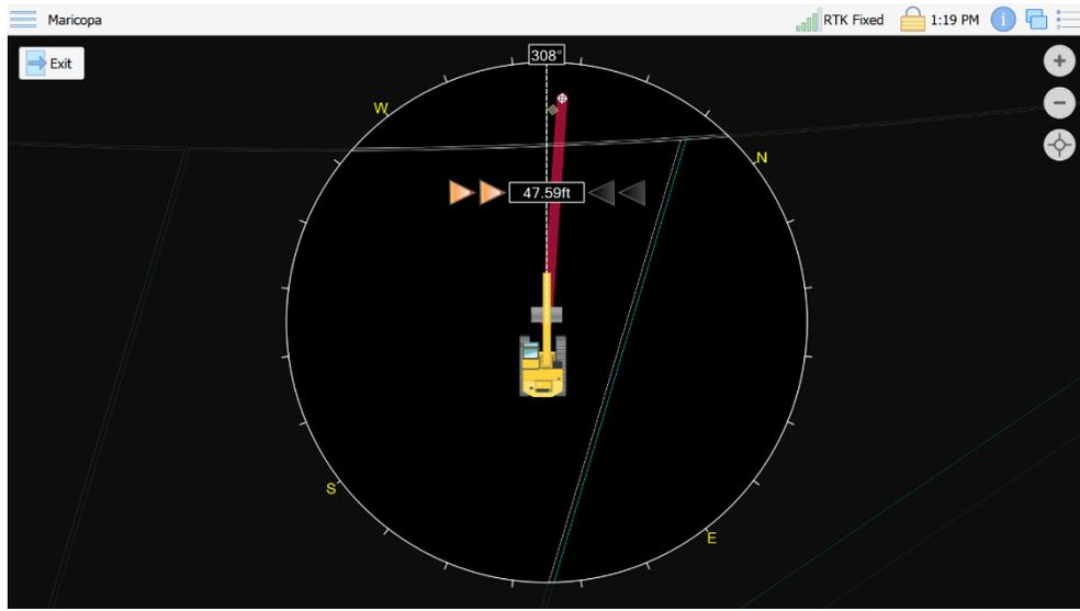
As the machine is driven closer, the screen begins to zoom in automatically.
