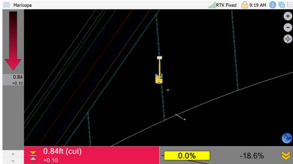
To add a specific vertical offset, or adjust the step size, click and hold the Cut/Fill arrow. The following dialogue window appears:
