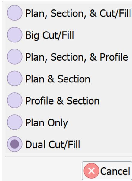
The **Dual Cut/Fill** screen displays a cut/fill value on both sides of the bucket.
