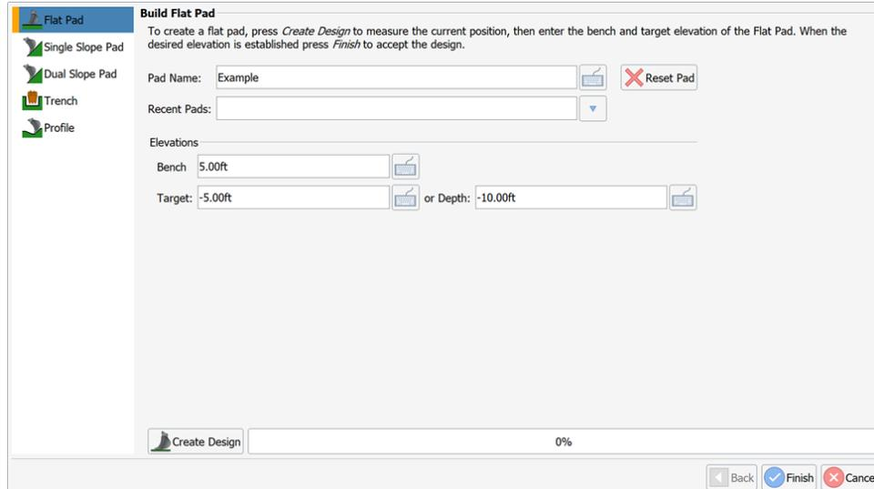
The screenshot shows the 'Build Flat Pad' dialog box. On the left is a sidebar with icons for 'Flat Pad', 'Single Slope Pad', 'Dual Slope Pad', 'Trench', and 'Profile'. The main area contains the following fields and controls:
