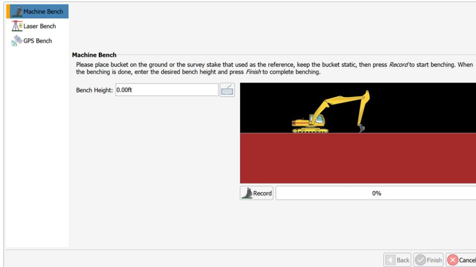
You can set the cutting edge on a benchmark, **Machine Bench – to GPS Bench**. Type the **Bench Height** and click **Record**.
