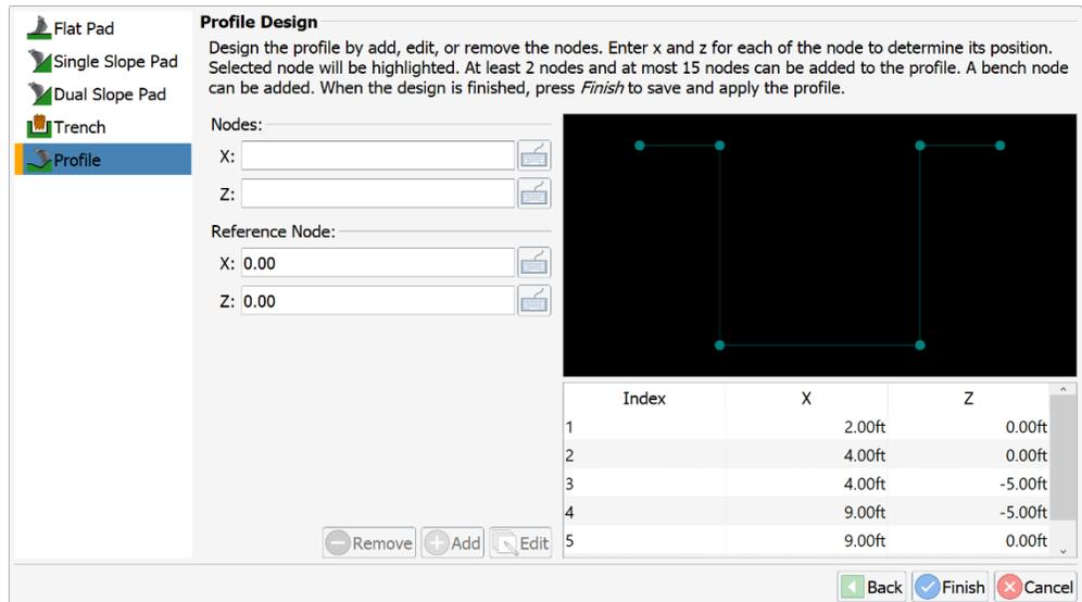
Enter a **Reference Node**. The **Reference Node** is only for reference on the screen and is not part of the profile. Build the **Profile** by entering the nodes and click **Add**.
