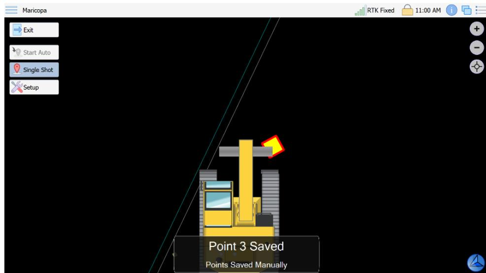
In the example above, locate the orange square on right side of cutting edge. This is the point just stored. Note it is on the right, as you set up in settings (**Point of Interest**), and the message reads “**Point 3 Saved**”, because you started with 3 (see following screenshot). If for example, you start with 50, the message would read “**Point 50 Saved**”.
