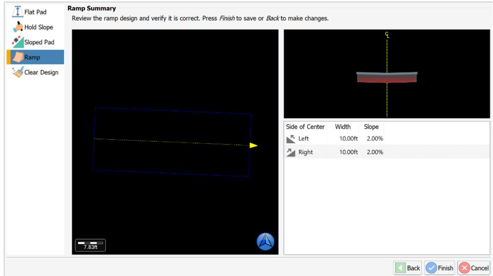
The screenshot shows the 'Ramp Summary' dialog box. On the left is a toolbar with icons for 'Flat Pad', 'Hold Slope', 'Sloped Pad', 'Ramp', and 'Clear Design'. The 'Ramp' icon is highlighted. The main area contains a top-left view of a ramp design on a black background with a yellow dashed centerline and a blue arrow pointing right. A scale bar at the bottom left of this view shows '7.83ft'. To the right is a 3D perspective view of the ramp. Below these views is a table with the following data:
