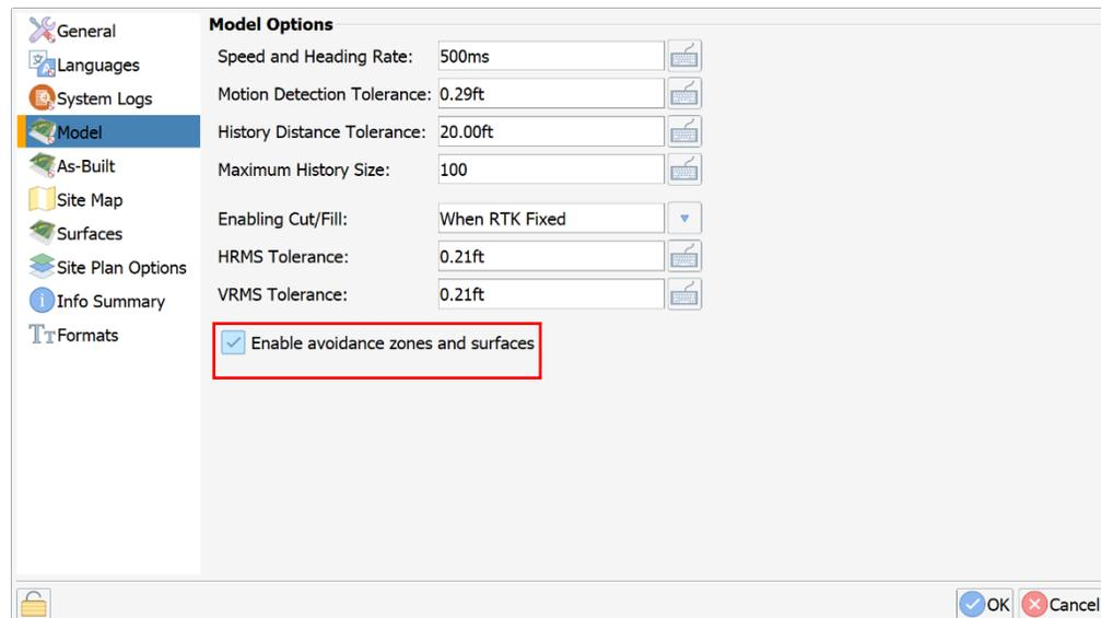
Click to select the checkbox to select **Enable avoidance zones and surfaces**. If the module is built with avoidance zones, an alarm will sound when entering those zones.
