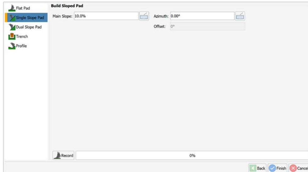
Click **Record**. The **Offset** is the difference between the current machine azimuth (coming from the GNSS receiver) and the azimuth you type in. If you do not have a dual antenna GNSS receiver connected, azimuth will be 0.
