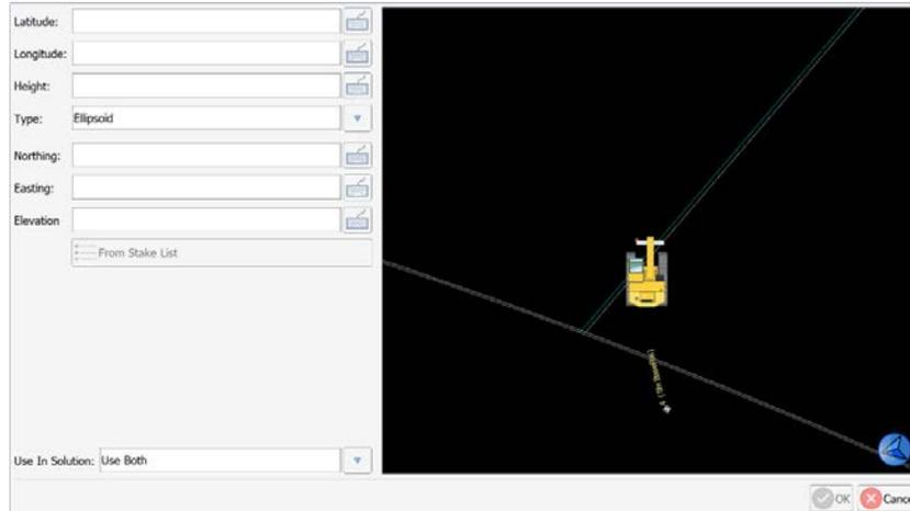
The **From Stake List** button-allows the user to select a control point from the stake list.
