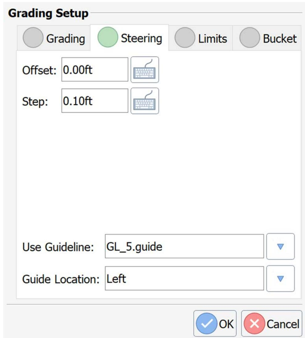
The **Grading Setup** dialog box features four tabs: **Grading**, **Steering** (selected), **Limits**, and **Bucket**. The **Steering** tab contains the following controls:
