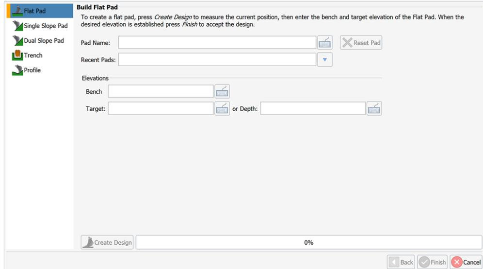
Use **Flat Pad** to create a surface at a set elevation:
