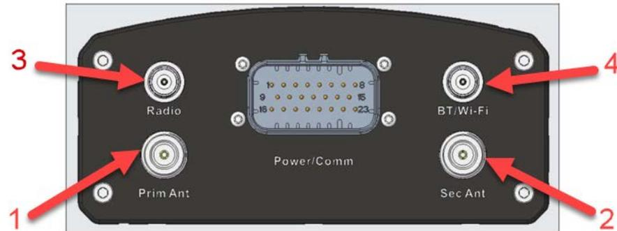
**Figure B-2: VR1000 pin-out assignments**
