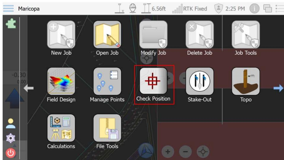
**Check Position** checks the accuracy of your GNSS receiver. Place the receiver onto a control point, select the point from the loaded file, and click **Check**. Your current GNSS position is read and averaged, and the deltas to that point are checked.
