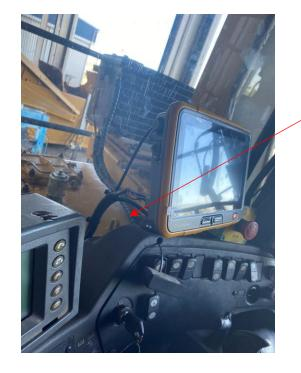
Cables run behind here to the pillar. CAN cable comes around to the back of the chair. The VR500 cable and 4G cable goes up the pillar into the roof lining. Yellow Y cable goes to the left and sits behind the screen on the dash.
