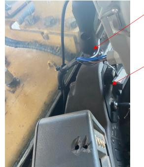
4G cellular cable, runs outside to the magbase antenna. Use grommet or silicone to plug the hole around the conduit.
