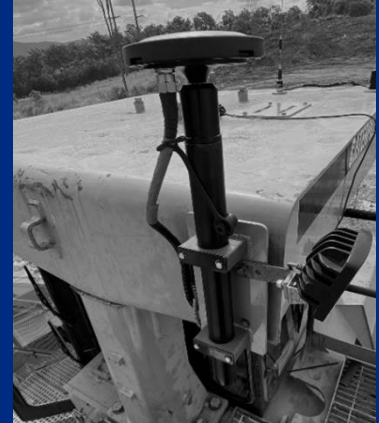
CAT D10R Dozer – A46 Antenna – RER brackets
