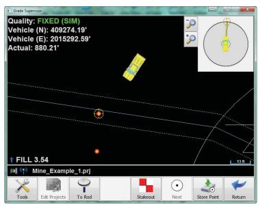
The direction compass in the top right will guide you to the point. The machine is located on the center of target. The point you are staking out will be shown on the outer circle of the compass and relative to the direction needed to reach the point. As you approach the point, the bullseye will move in closer to the machine, the arrow will turn green and become larger. Once you are over the point, the bullseye will center of the machine's referenced cut/fill location.
