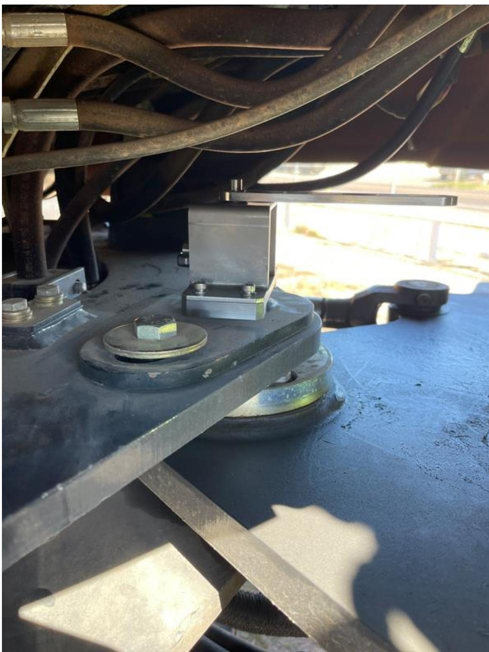
**Figure 2-14: Encoder with Bracket**
