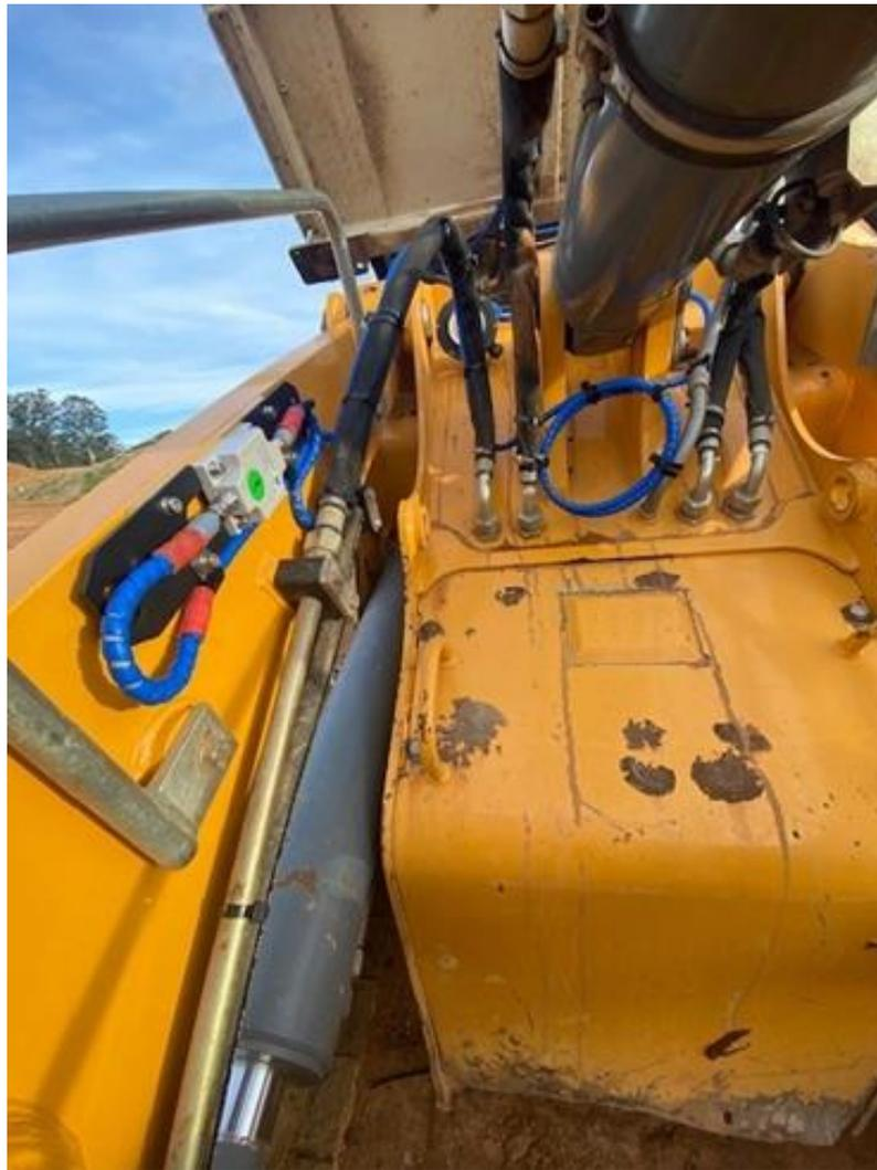
**Figure 2-9: Boom sensor installed on the inside of the boom**
