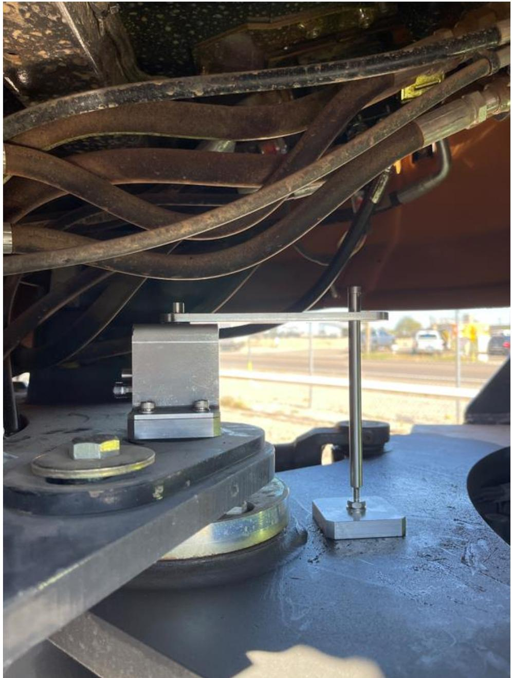
**Figure 2-15: Encoder Shaft**
