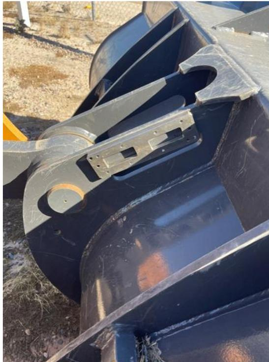
**Figure 2-7: Bucket Sensor Mount**
