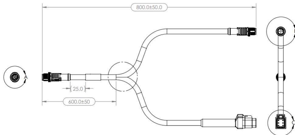
**Figure 4-3: Cable schematic for P/N: 051-0426-10 (IronTwo)**
