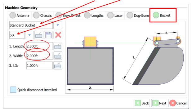
Change the length and if needed, the width of the bucket. Using a tape measure, measure the distances as shown for 1 & 2. Do not touch 3. L3. To make the changes, simply click in the boxes circled. Once complete click *Next > Next & Finish* to save.
