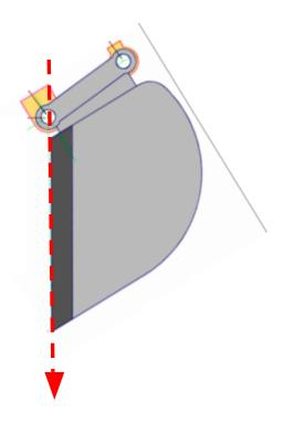
Highlight the bucket sensor and click *Calibrate*. Once the bar and counted to 100%, click *OK*.
