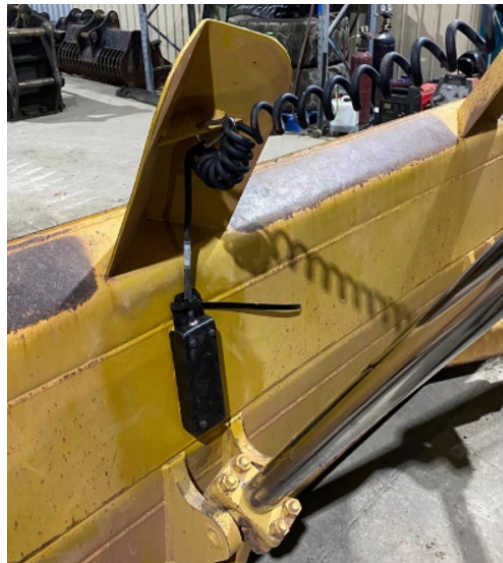
Figure 2-6: Horizontal Sensor and Chassis
