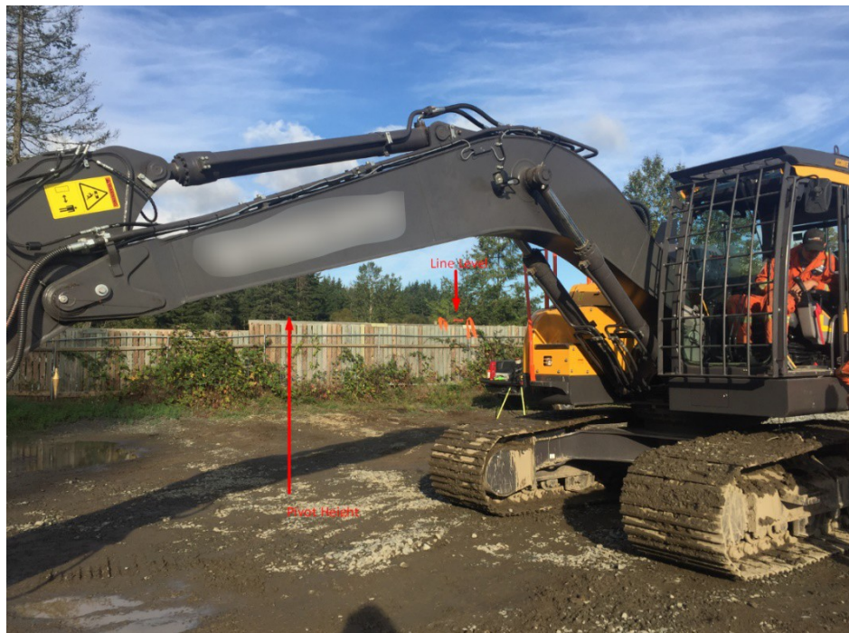
Figure 3-2: Measuring the pivot height
