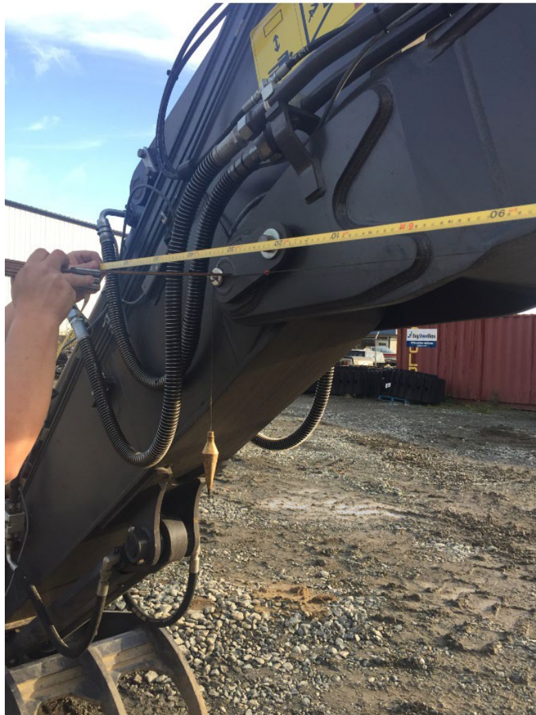
Figure 3-3: Measuring the boom pin to stick pin
